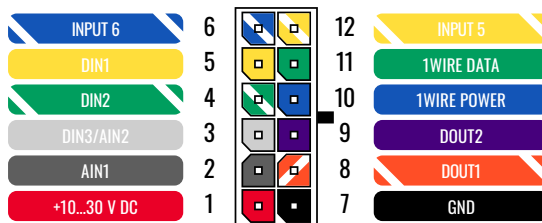
FMB110 2x6 socket pinout
